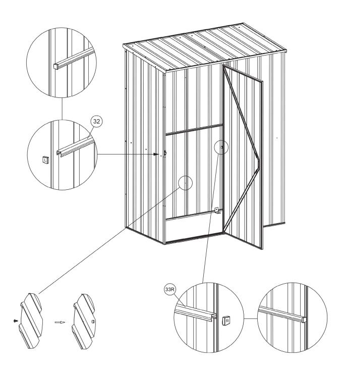
The door can be hinged on the opposite side as well. Align the door with the edge and make the holes using a cordless drill. Remove the pins from the hinges and reverse their direction before you attach the door. If you are concerned about the visibility of any pre-drilled holes, you can fill them with rivets. Perform the same procedure for the pad bolt.
