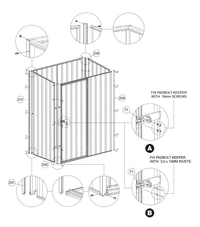
Now fit the bolt down kit as per the diagram below. Strengthen the mid wall braces by applying part 72 (mid wall brace bracket) on each corner if necessary.
