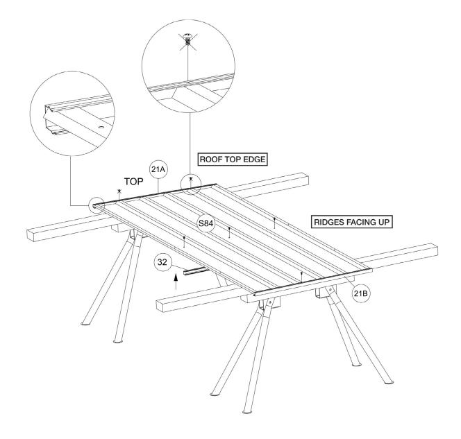
**Tip:** If panel and screw holes do not line up, try pulling panel to match up holes.
